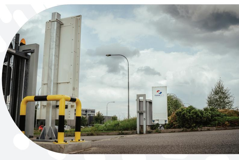
The detection gate is equipped with two 40 L scintillation detectors that can be used for quick and easy inspection of trucks and cars transporting scrap metal. The high sensitivity of the detection system ensures high reliability of detecting a potential source of ionizing radiation.
